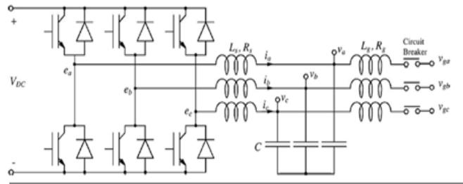
Fig 1: Power part of a synchronverter.
