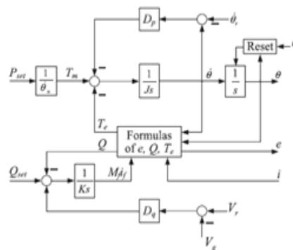
Fig :2 Electronic part (controller) of a synchronverter, where the provision of the frequency reference  $\theta^*r$  , the phase reference  $\theta^r$  , and the voltage reference  $V_r$  , normally via a dedicated synchronization unit, is not shown.
